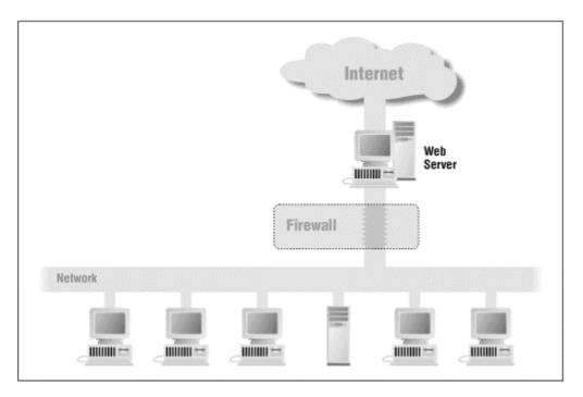
Figure 1.4. A web server located outside a firewall
